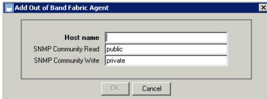
Figure 14. Adding information for a Brocade switch
